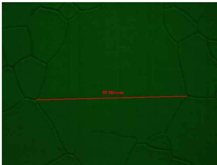
Figure 6. Micrograph of detector prototype for Colorado-Indiana experiment, showing crystal grain 90 \mu\text{m} wide.
