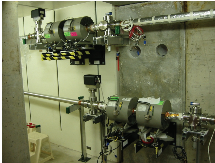
Figure 7. Focusing Solenoids in the Supply Line (Top) and the Transfer Line (Bottom) of the Electron Cooling System in the MI-31 Connecting Enclosure
