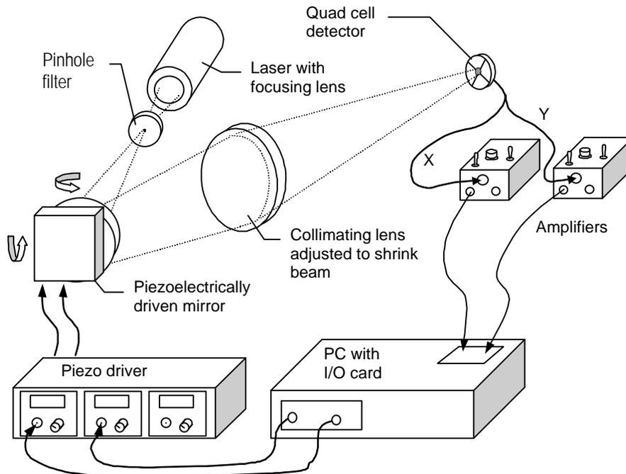
Figure 3: Experimental setup for investigating digital feedback system.
