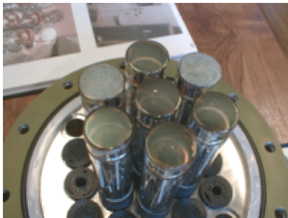
Figure 8. The same PMTs as in Fig. 7, after the first immersion in hot water for up to 40 days (equivalent to 17 months at 28°C). Notice that the four “clear” PMTs shown in Fig. 7 became “milky.”
