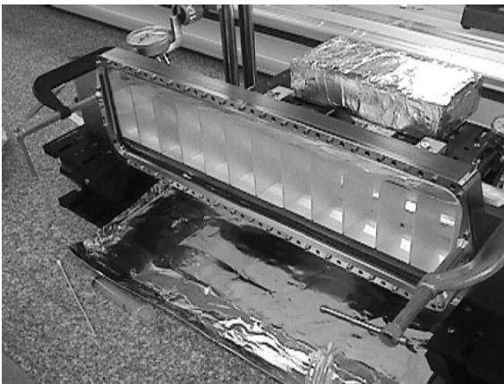
Figure 28. End view of the window of a bar box showing the window-frame, fused-silica window and twelve wedges.
