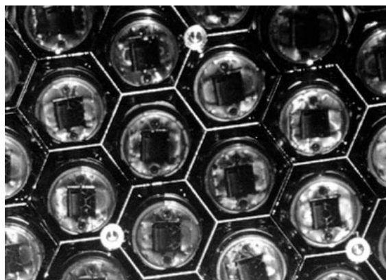
Figure 39. PMTs and rhodium-plated light-catchers in the SOB.
