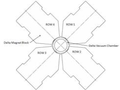
Figure 2: Arrangement of the Delta magnet blocks around the vacuum chamber, which has an ID of 5.08 mm and an OD of 6.4 mm, resulting in a 0.66 mm wall thickness.
