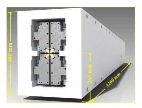
Figure 1: Layout of the 3.2-m long LCLS Delta undulator.
