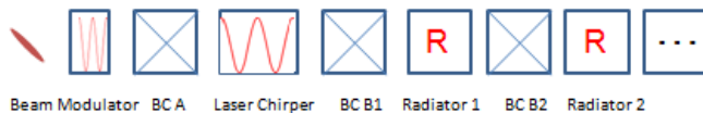
FIG. 1: A schematic plot of the lattice layout of the modulation compression scheme.
