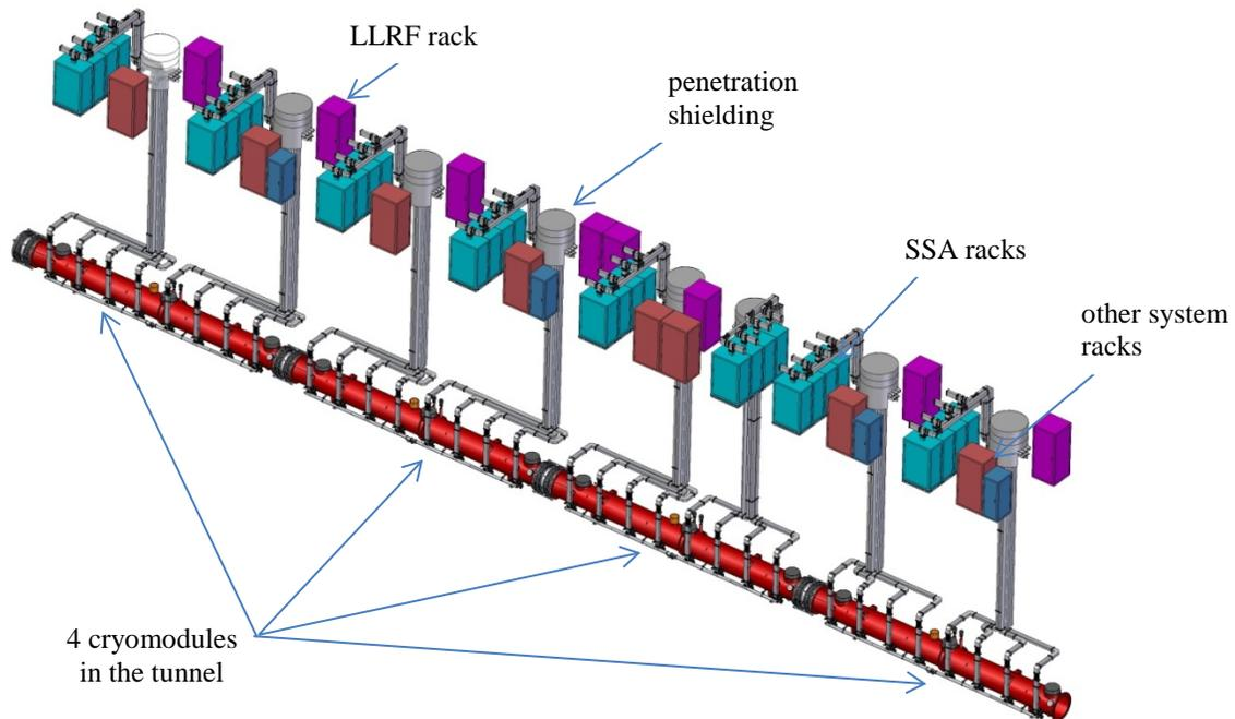
Figure 2: Gallery and tunnel layout of eight penetration or four cryomodule section of LCLS II
