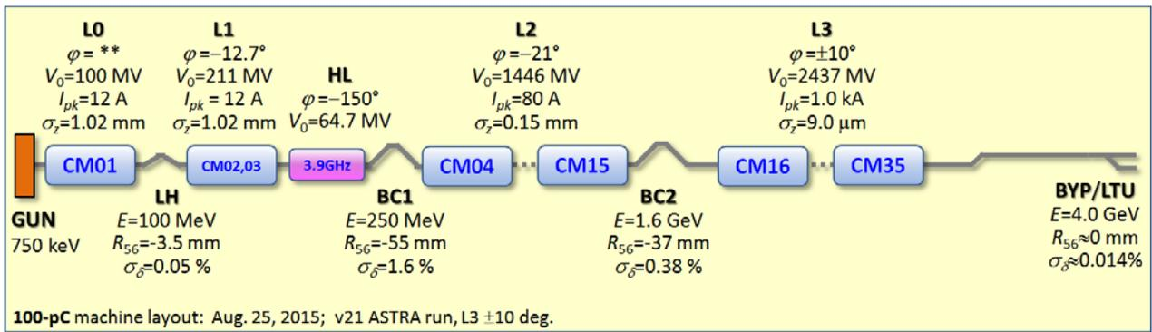
Figure 1: LCLS II Beamline Diagram
