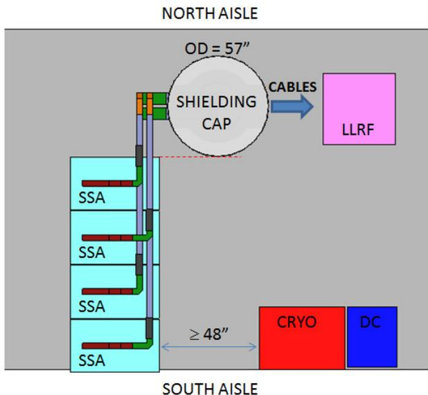
Figure 3: Projection of a single penetration layout.
