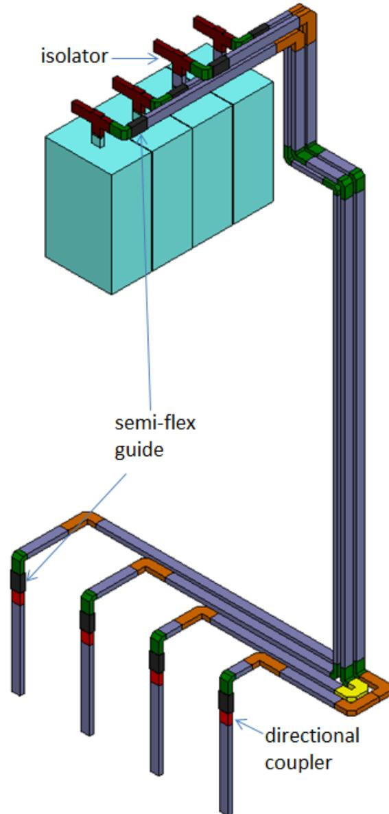
Figure 4: Waveguide system layout from four L-band SSAs to four cavity couplers through one penetration.
