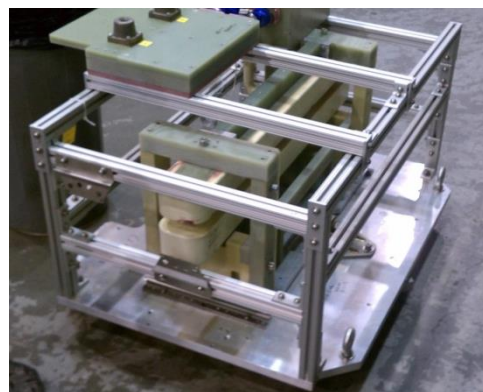
Figure 1b: Original Al frame and baseplate kicker magnet
