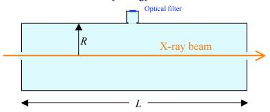
Fig.1 Schematic of the photoluminescence cell. The visible and UV light created in the cell passes through the optical filter and hits a detector (not shown). At a given fill pressure and X-ray energy  $E_X$  the detector signal is the measure of the pulse energy Q.
