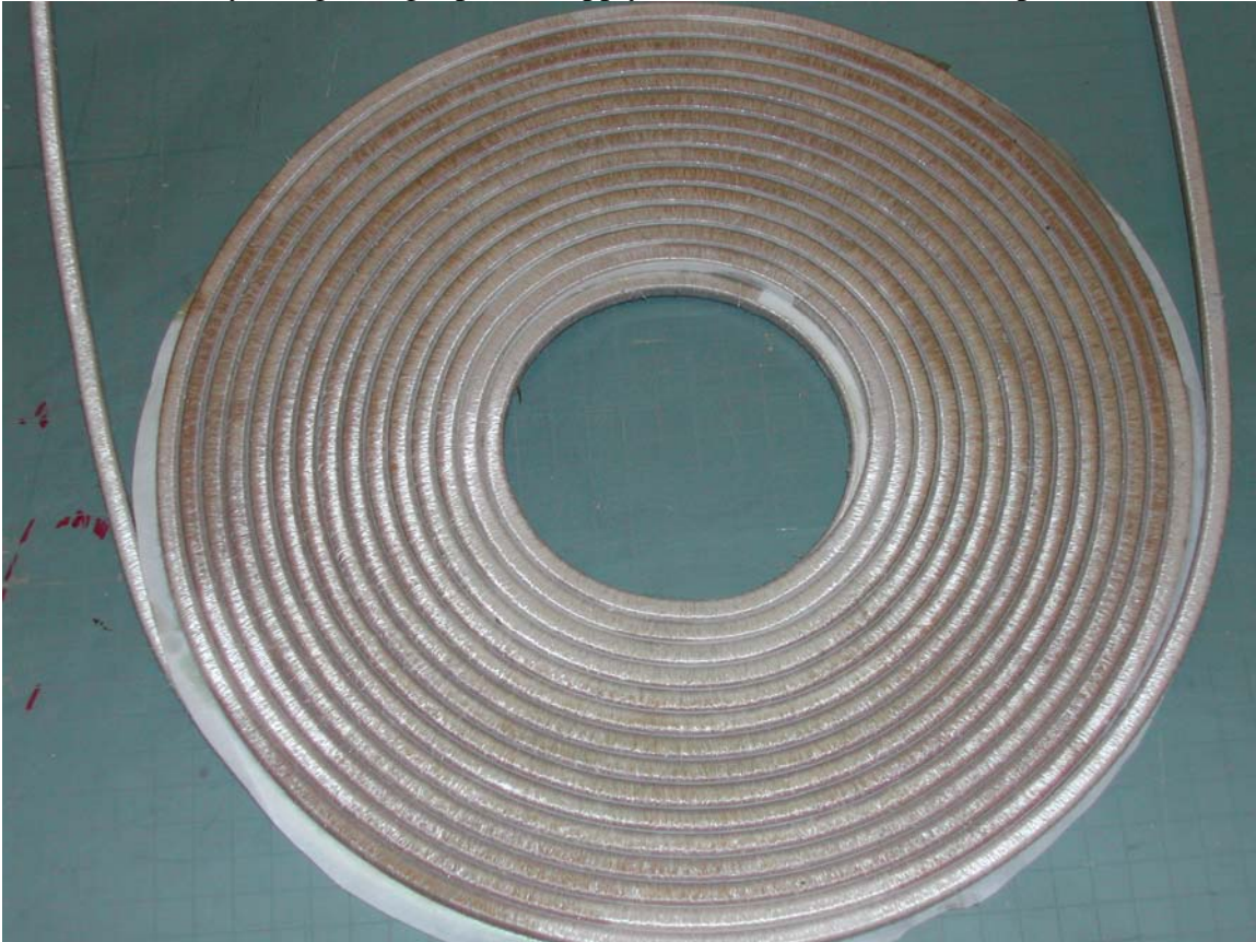
Figure 4: The two layer pancake coil prior to potting.
