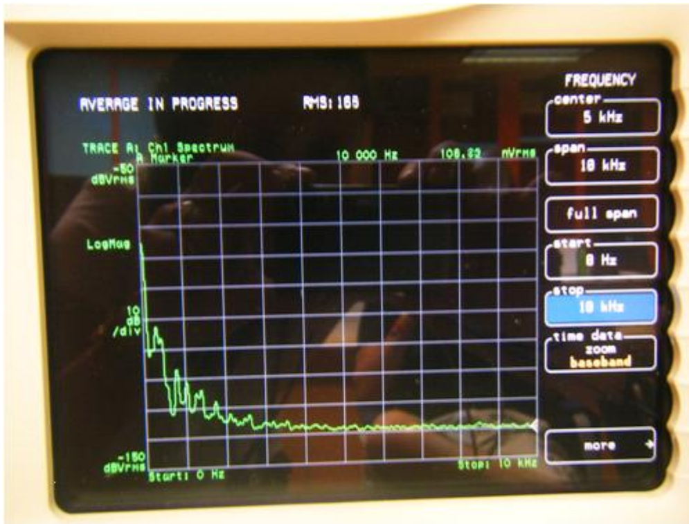
Figure 5. The spectrum analyzer displays a noise plot that resembles a 1/f plot.
