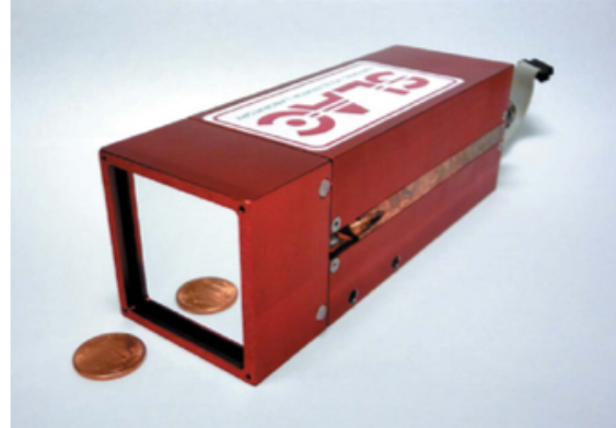
Figure 5. 7 (right) ePix camera. This is the assembly used for the different ePix detectors.
