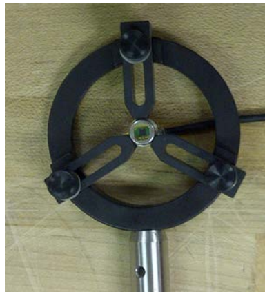
Figure 4: Pyroelectric single cell detector mounted on a holder.
