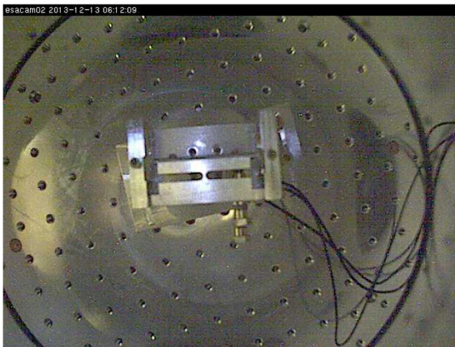
FIG. 1. crystal stage inside the scattering chamber (beam enters from the top of the figure)
