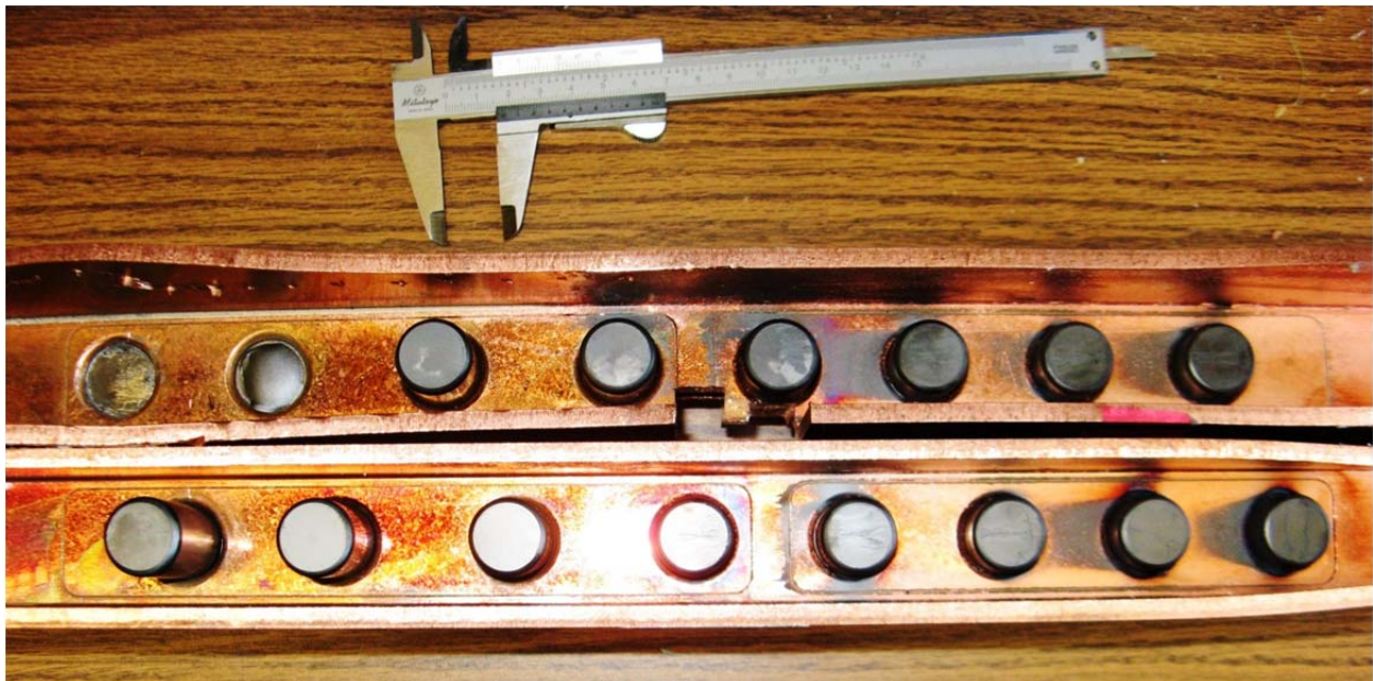
Figure 6 Cut-away view of the Nihon Koshuha Co. Dry Vacuum Load after breakdown: side by view of narrow walls
