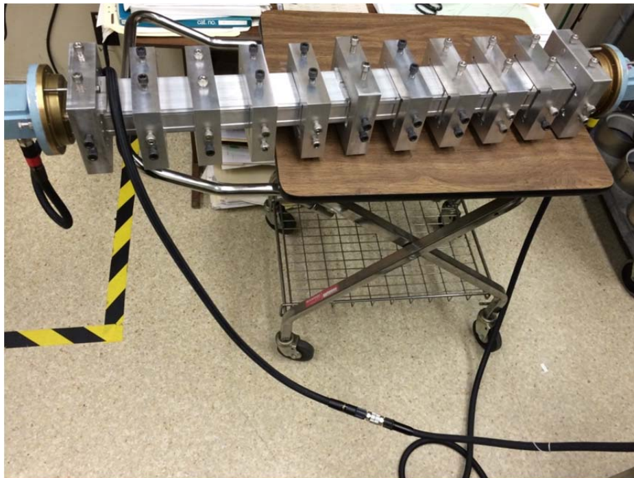
Figure 22 Coated waveguide at LLRF measurement
