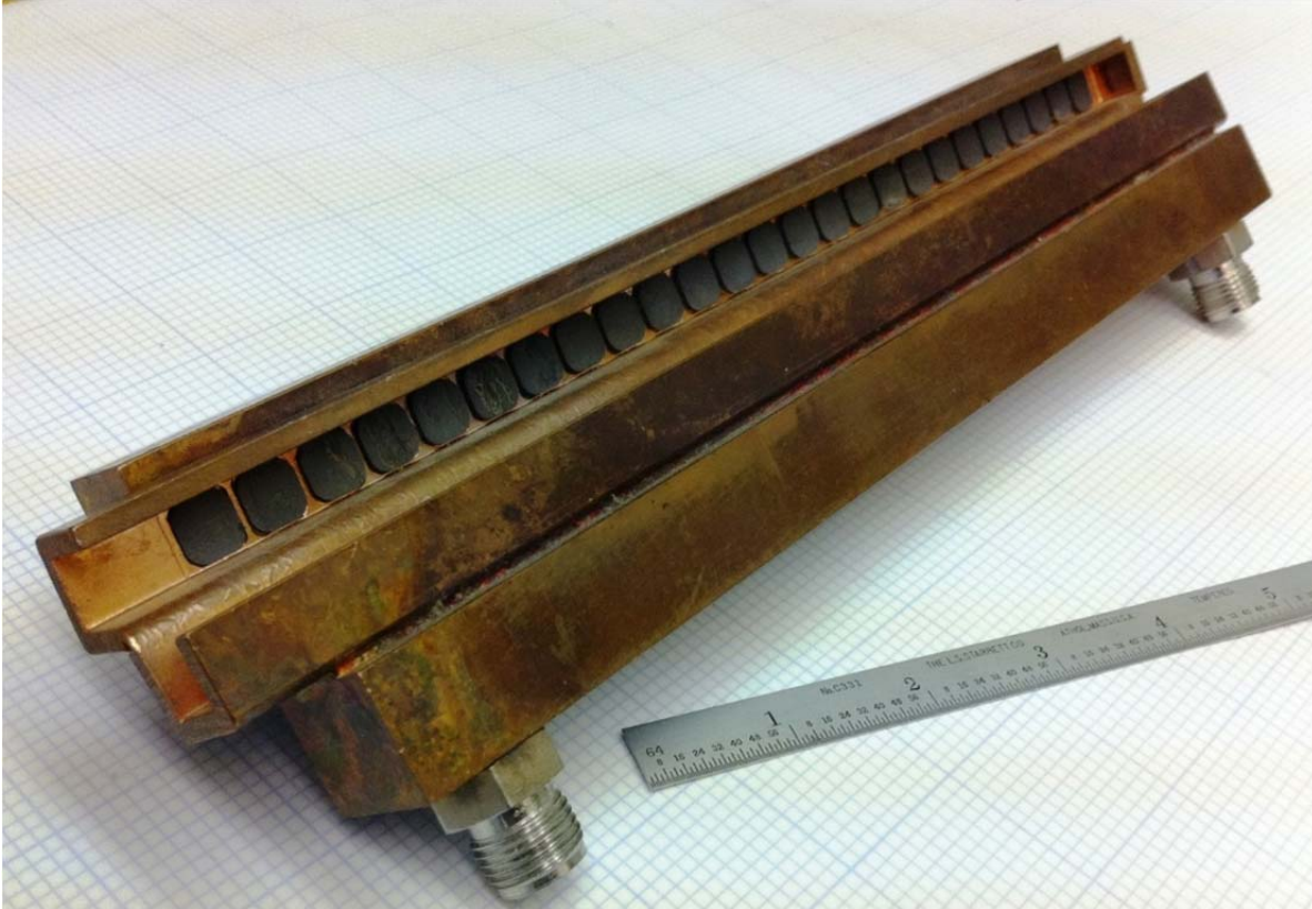
Figure 4 Vacuum Dry Load with lossy ceramic wedges
