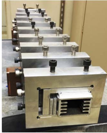
Figure 29 Cross section of the RF load end is close to the frequency cutoff. Wave group velocity on this end is close to zero
