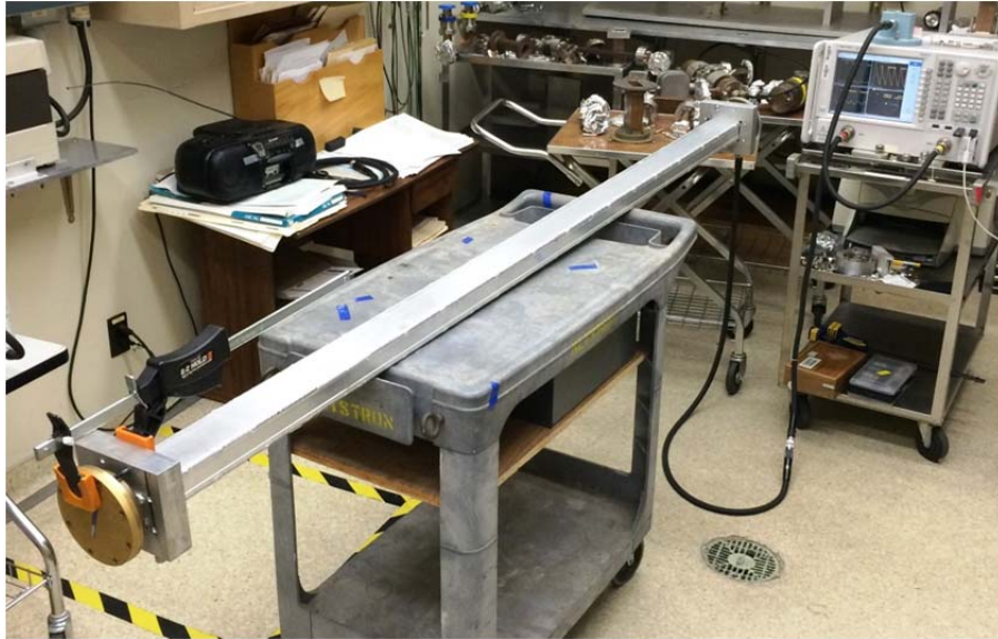
Figure 23 Welded waveguide with absorption layer
