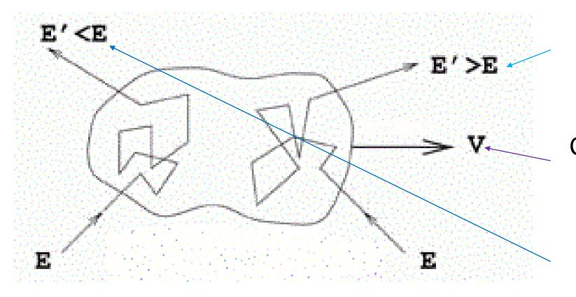
head-on collision; particle gains energy
