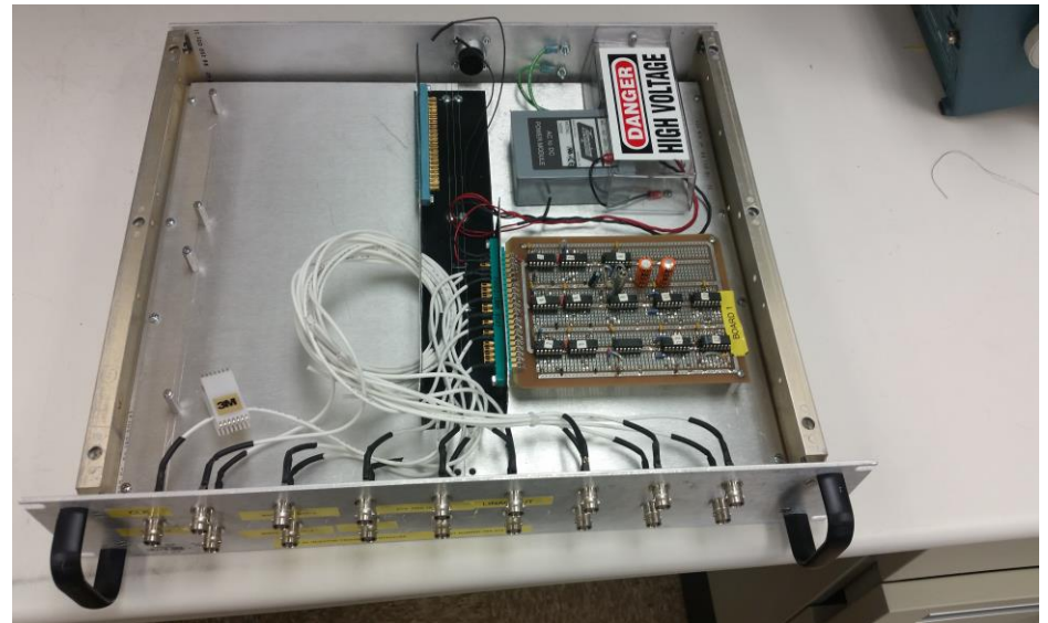
Fig. 4 switching circuit prototype in chassis
