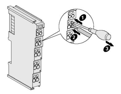
Up to eight connections enable the connection of solid or finely stranded cables to the Bus Terminals. The terminals are implemented in spring force technology. Connect the cables as follows:
