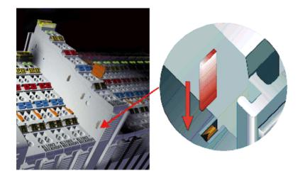
Note that, for reasons of electromagnetic compatibility, the PE contacts are capacitatively coupled to the mounting rail. This may lead to incorrect results during insulation testing or to damage on the terminal (e.g. disruptive discharge to the PE line during insulation testing of a consumer with a nominal voltage of 230 V).
