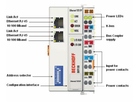
The BK9100 Bus Coupler connects Ethernet with the modular, extendable electronic terminal blocks. One unit consists of one Bus Coupler, any number from 1 to 64 terminals and one end terminal.
