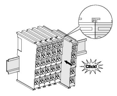
The Bus Coupler and Bus Terminals are attached to commercially available 35 mm mounting rails (DIN rails according to EN 50022) by applying slight pressure:
