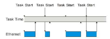
If, after the task time has elapsed, an Ethernet telegram has still not arrived at the PC, only reaching it after the next task has started, then TwinCAT will continue to work with the old input data. In addition, the *MissedCnt* counter is incremented.
