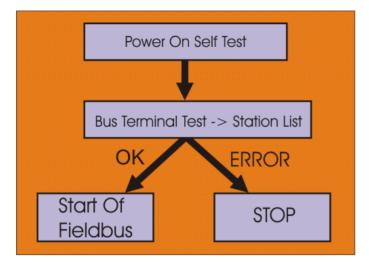
The Bus Coupler can be made to enter the normal operating state by switching it on again once the fault has been rectified.
