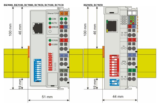
The total width in practical cases is composed of the width of the Bus Coupler, the width of the bus terminals in use and the KL9010 Bus End Terminal. Depending on function, the Bus Terminals are 12 or 24 mm wide. The front wiring increases the total height of 68 mm by about 5 to 10 mm, depending on the wire thickness.
