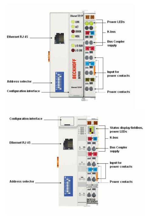
The BK9000 and BK9050 Bus Couplers connect Ethernet with the modular, extendable electronic terminal blocks. One unit consists of one Bus Coupler, any number from 1 to 64 terminals and one end terminal. The BK9050 compact Bus Coupler is a cost-optimized version with compact housing. With the K-bus extension, up to 255 Bus Terminals can be connected.
