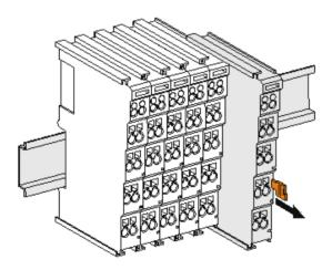
Each terminal is secured by a lock on the mounting rail, which must be released for disassembly:
