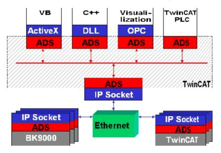
The ADS protocol runs on top of the TCP/IP or UDP/IP protocols. It allows the user within the Beckhoff system to use almost any connecting route to communicate with all the connected devices and to parameterize them. Outside the Beckhoff system a variety of methods are available to exchange data with other software tools.
