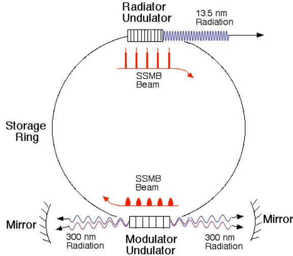
Figure 3: Schematic of the proposed SSMB device. The two mirrors are needed only to reduced the required seed laser power. Otherwise it is to be avoided to minimize any storage ring FEL accumulation.
