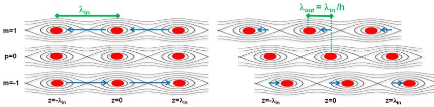
Figure 2: Staggered buckets as viewed at the modulation point (left), and as viewed 1/3 around the ring ( $h = 3$ ) (right). The projected beam distribution at the 1/3-location is microbunched at the 3rd harmonic of the modulation frequency.
