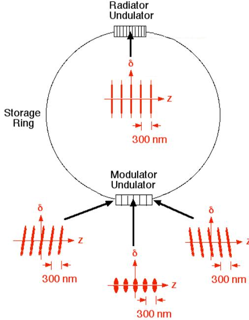
Figure 4: Schematic of longitudinal phase space distribution of the microbunches at various locations around the storage ring.
